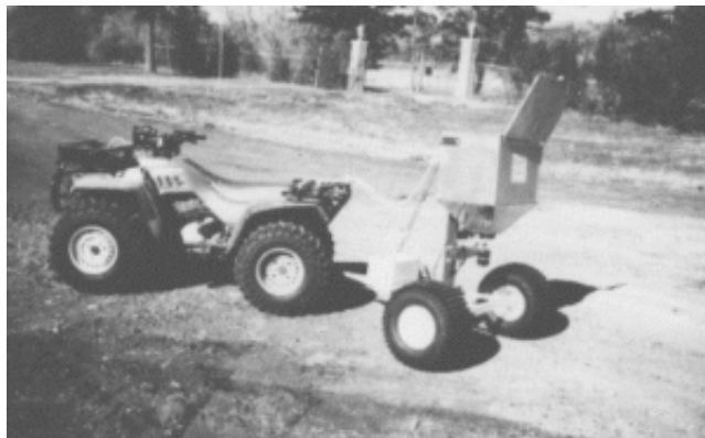
(Figure 6. Four-wheel ATV's are used to apply granular fertilizer between rows of plantations)
