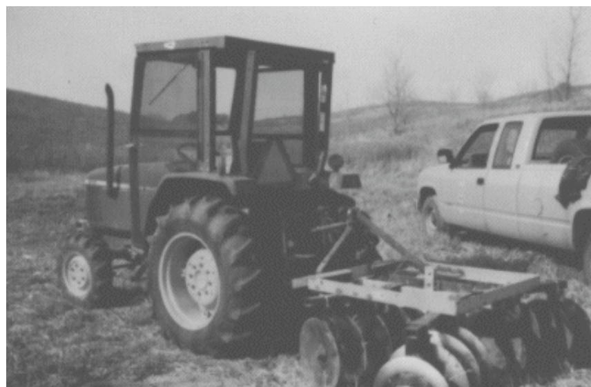
(Figure 5. Narrow four-wheel drive tractors are used for between-row operations)
