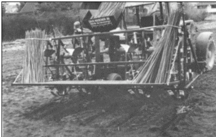
(Plate 1. Salix Maskiner Four Row Step Planter From Sweden) Cuttings are planted at around 10,000/ha into a pre-prepared seedbed using a mechanical planter. A modified cabbage planter can be used although other mechanized techniques have been developed such as the Salix Maskiner step planter from Sweden .
