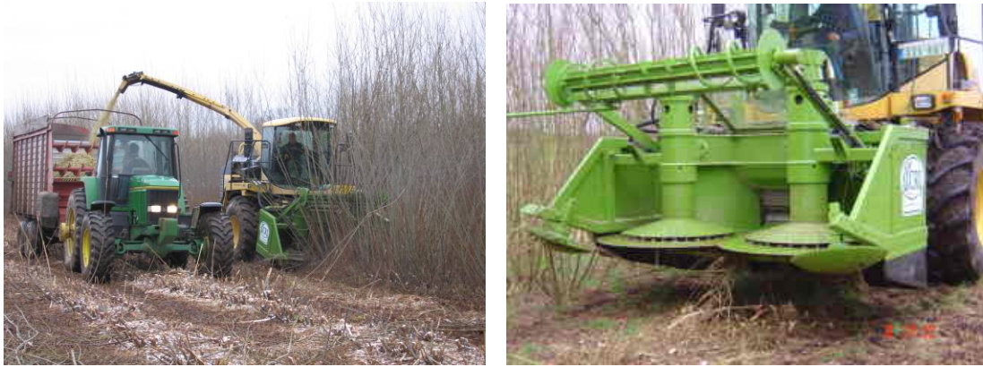
Figure 2. Harvesting willow biomass crops with a New Holland FX45 forage harvester and a specially designed Coppice Resources Ltd. (CRL) willow cutting head in NY during fall 2006 and a close up view of the CRL willow cutting head.
