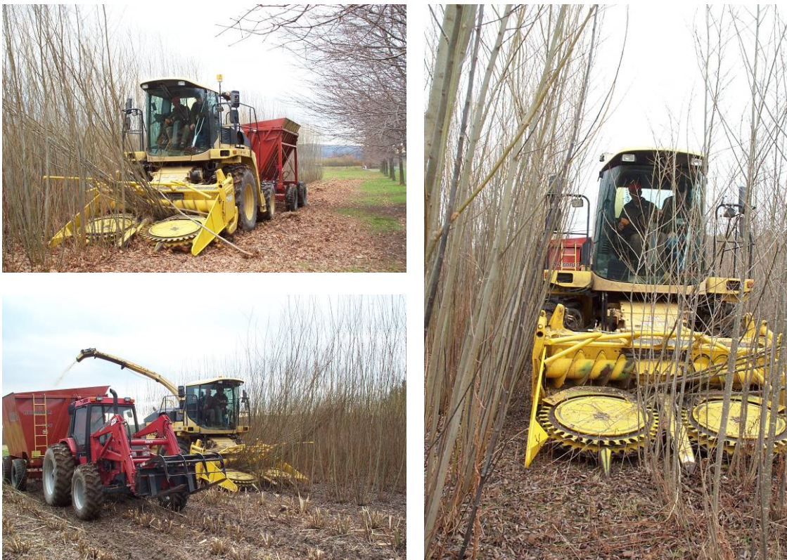
Figure 1: New Holland FX45 forage harvester with a modified row independent corn head harvesting 3-year-old willow biomass crops during field trials in December 2004 and January 2005 at the SUNY-ESF Genetic Research Station in Tully, NY.
